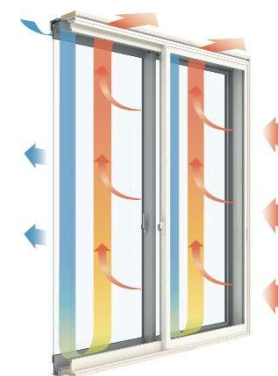
DI (Dynamic Insulation) Window
